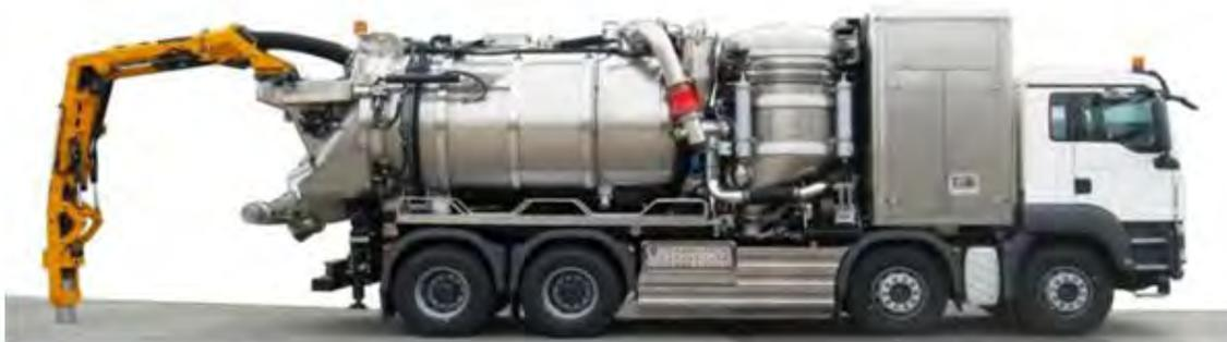
**Tank / Debris - capacity 11 cubic metres**
