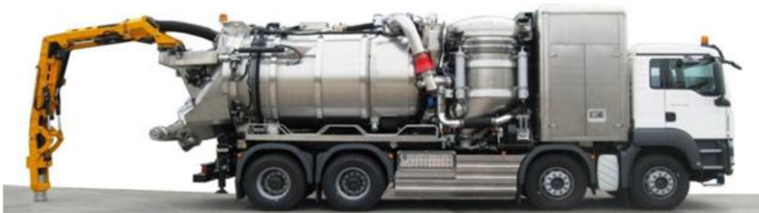
Vacuum Loader - Cap Bora Excavation Unit
