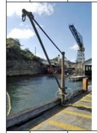
An early hand operated jib crane apparently added to the 1945 wharf. Its former location and use (it is significantly older than the wharf on which it was located) and history are not known. The crane is now beneath wharf debris on the floor of the harbour after the collapse of this section of the broadside wharf.
