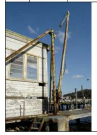
A jib crane with braces located on a small section of wharf near the repair workshop. The crane appears to date from the 1945 period.
