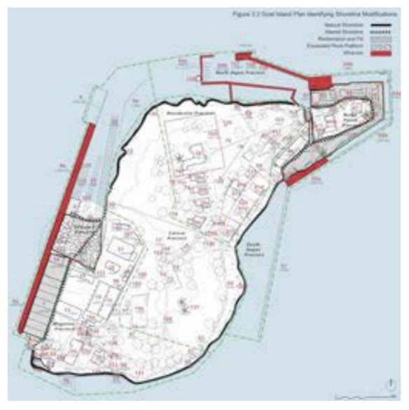
Figure 3.3 Plan of Goat Island showing the extent of modified and non-modified shoreline, areas of fill and excavation around the shoreline and the wharfs. This plan indicates that most of the shoreline remains in intact or with only very minor modifications to the natural edge. This plan is based on the 2007 aerial photograph and it is noted that sections of wharfs 4a, 4b, 5 and 51 and wharves 52b, 54c, 55a and 55b have collapsed and been removed.
