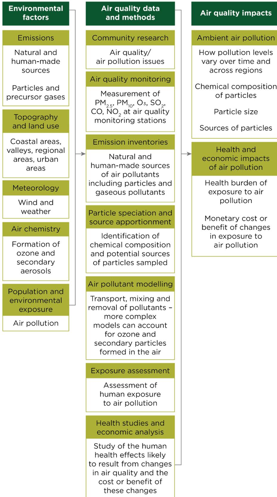
**Figure 2** Data and methods used in this study to understand air pollution and its impacts. CO = carbon monoxide; NO<sub>2</sub> = nitrogen dioxide; O<sub>3</sub> = ozone; PM<sub>2.5</sub> = particulate matter 2.5 micrometres or less in diameter; PM<sub>10</sub> = particulate matter 10 micrometres or less in diameter; SO<sub>2</sub> = sulfur dioxide.
