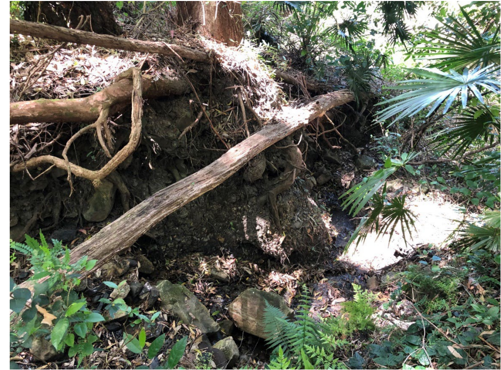
Terrain Unit 2 Photograph 14: Deep incised channels formed within the fill.
