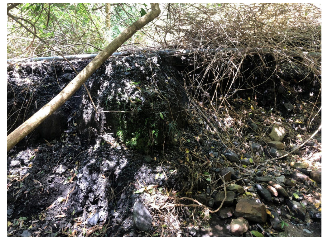
Terrain Unit 2 Photograph 12: View of coalwash like fill in the base of the gully network.
