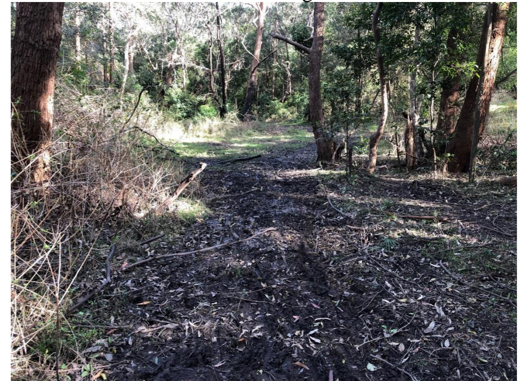
Terrain Unit 1 Photograph 4: Area of seepage observed at the toe of T1. Photo taken along Trail 6.
