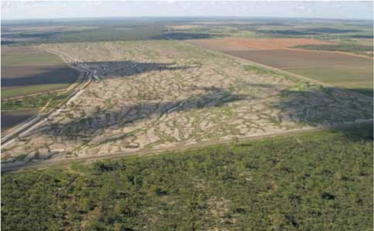
Photo 23 Development in the marshes located in the Marebone area. An identified floodway in centre has been cleared, and natural drainage patterns remain evident (W. Johnson).
