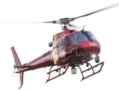
Helicopter with thermal imager and visual-spectrum camera for aerial survey of large animals. Gerhard Koertner/ DCCEEW
