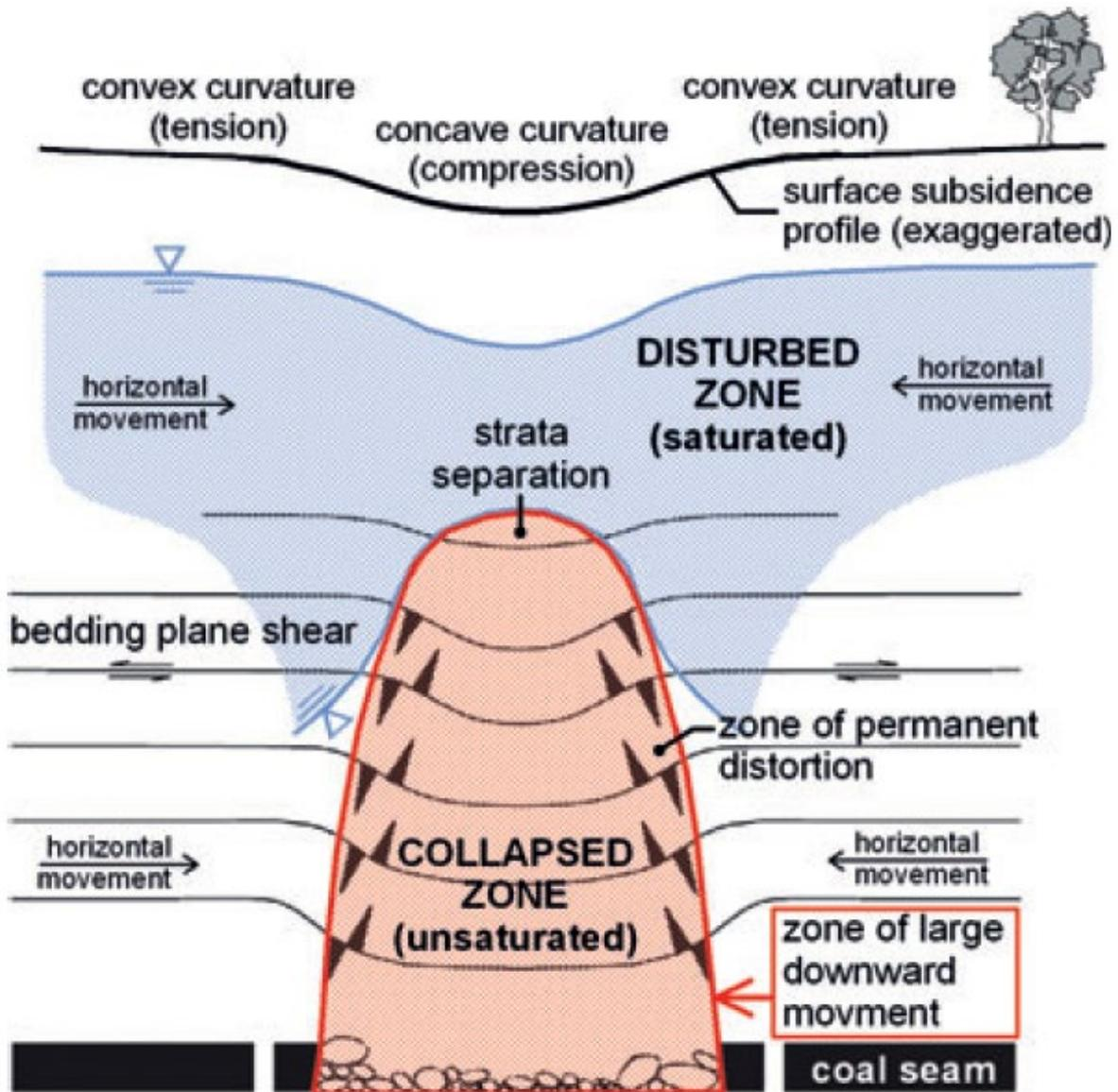
**Figure 3.2** Conceptual ground deformation model associated with Tammetta’s technique for predicting the height of complete groundwater drainage
