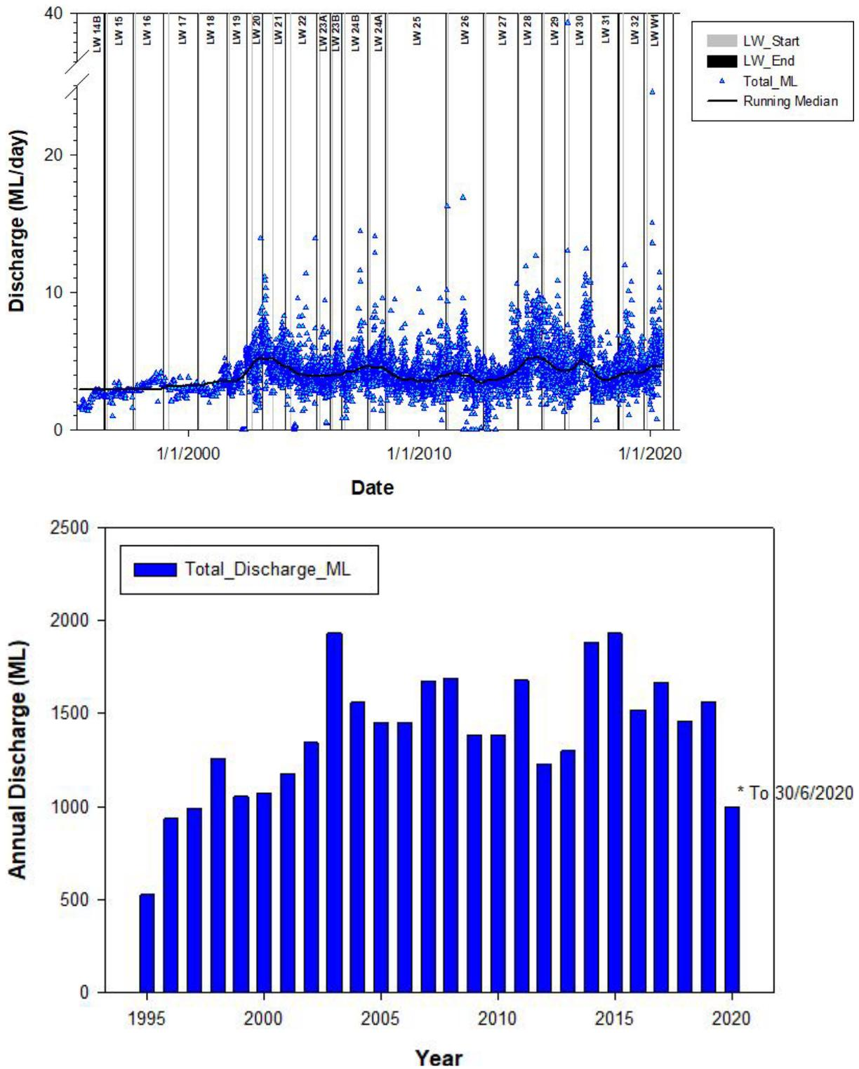
**Figure 3.12 Tahmoor Colliery discharge data 1995 to 30 June 2020; weekly/daily time series (above) and annual volume (below)**
