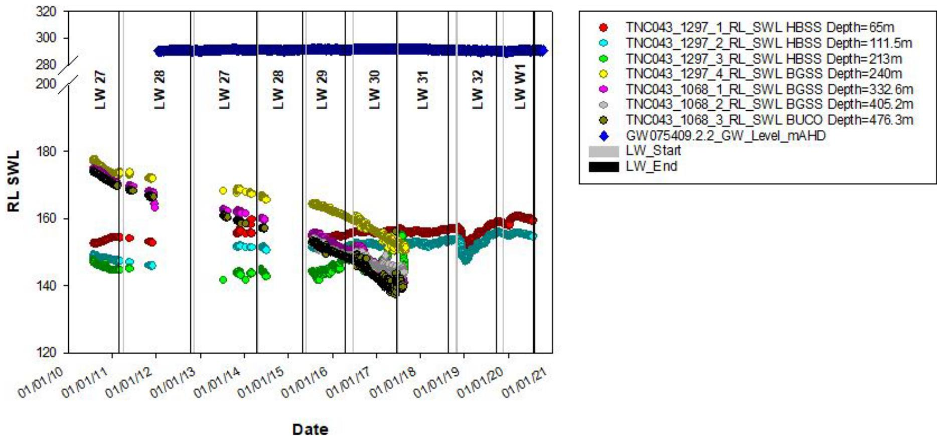
**Figure 3.11** Groundwater levels in TNC43
