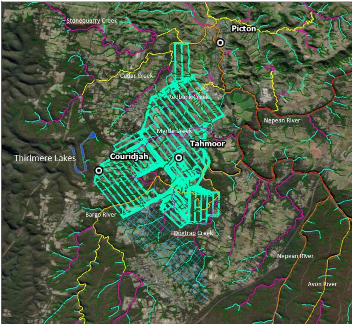
Figure 3.3 Longwall mining layout for Tahmoor Colliery relative to Thirlmere Lakes
