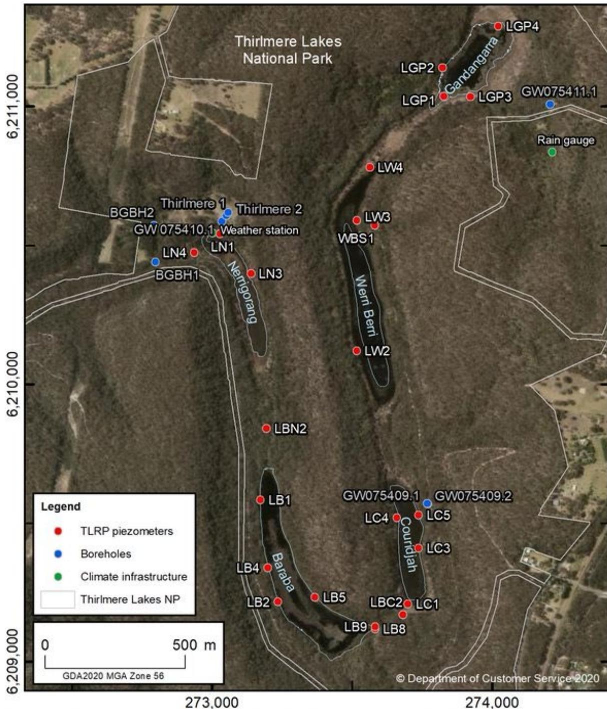
**Figure 7.2 Piezometer network established at Thirlmere Lakes**
